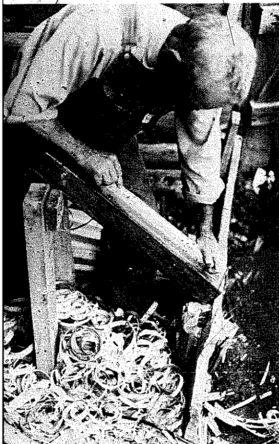
PLATE 340 Using a long-jointer, wood is planed from the edges of each stave until the angled edges fit the gauge.
