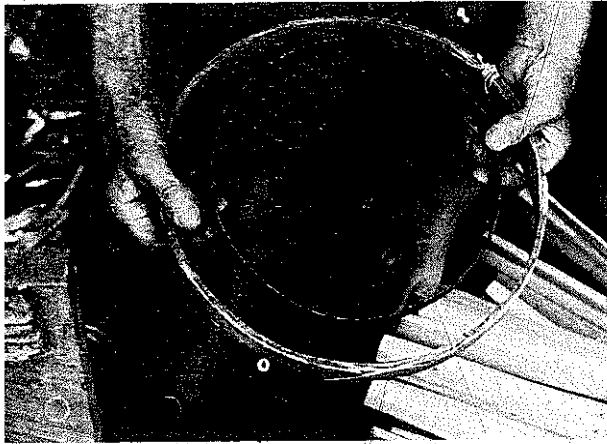
PLATE 343 Step 4: After staves are tapered and sides angled, Alex prepares to fit them into two temporary hoops.
