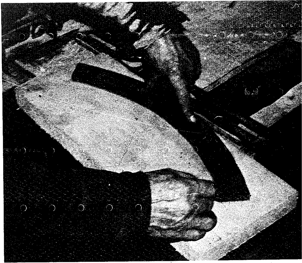
PLATES 90-93 A pattern is made for the wooden rim of the wheel (Plate 90), and the six felloes marked out on inch-and-a-half thick oak stock (Plate 91). Traditionally, these were cut out with a felloe saw (Plates 92-93 on p. 124).
