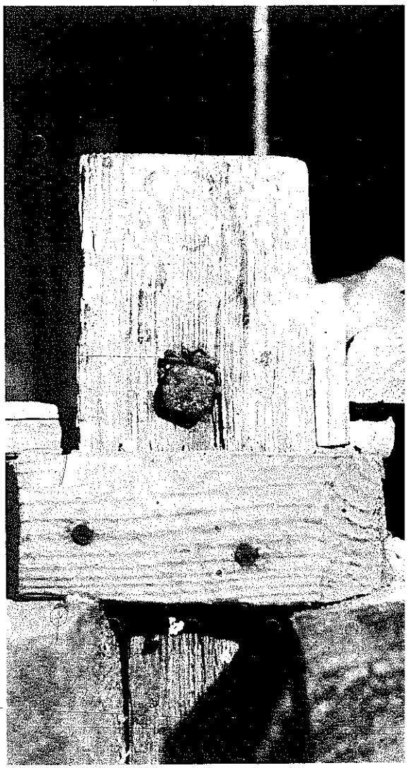
PLATE 181 Of special note are the two end pieces that hold the stock being turned. Rather than being mounted permanently on the vertical support beams, as on Minyard's lathe, these are cross-shaped pieces that slide back and forth between two horizontal beams (as shown here and in Plate 180 ) so that stock of varying lengths can be worked. The stock is held on either end by a metal spike driven through each cross-shaped end piece.
