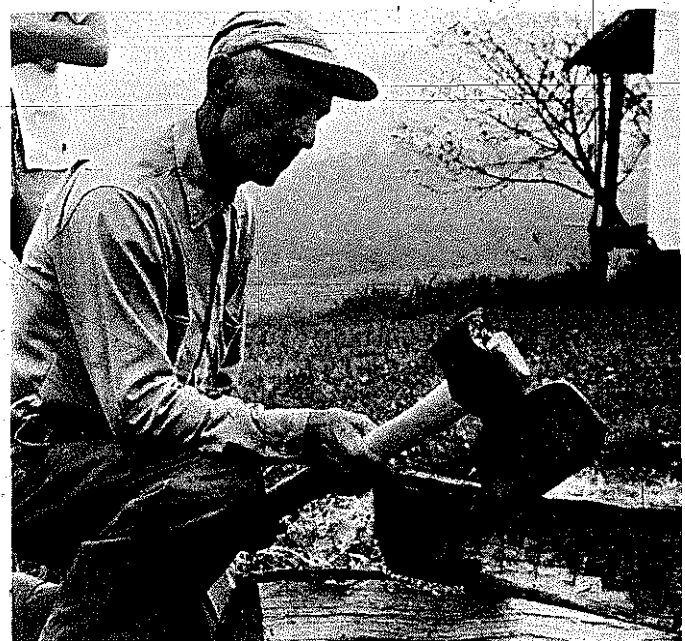
PLATE 15 Bill Lamb shows how to use a broadaxe. The vertical marks on the log were left by the scoring process.
