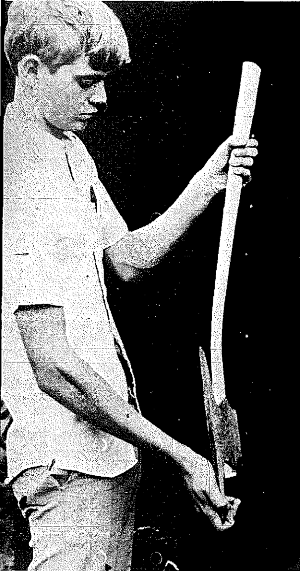
PLATE 16 As Paul Gillespie shows, a broadaxe has a curved handle to prevent the user's skinning his knuckles as he works.
